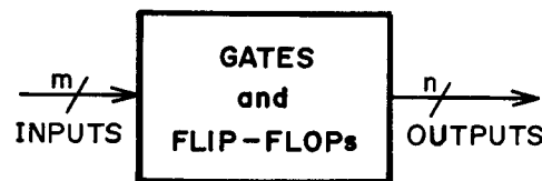
Fig. 2.1.2--Random Logic Sequential Circuit
