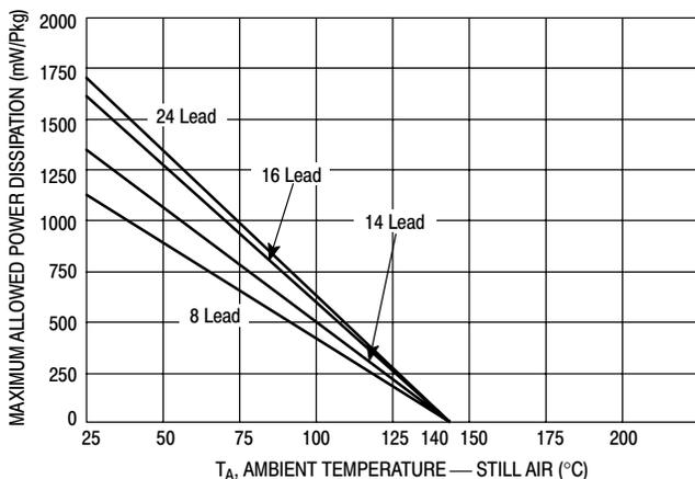
Figure 19. Ambient Temperature Derating Curves (Plastic Dual-In-Line Package)
