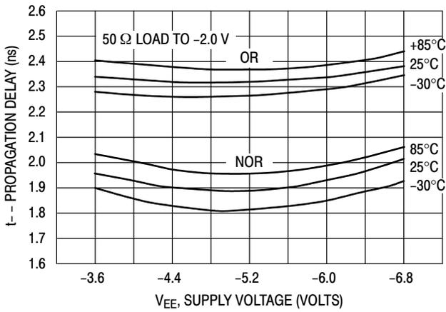
Figure 10. Typical Propagation Delay  $t_{--}$  vs.  $V_{EE}$  and Temperature (MECL 10K)
