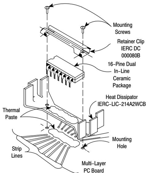
**Figure 26. MECL High-Power Dual-In-Line Package Mounting Method**
