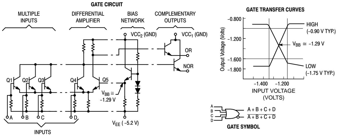
Figure 3. MECL 10K Gate Structure and Switching Behavior
