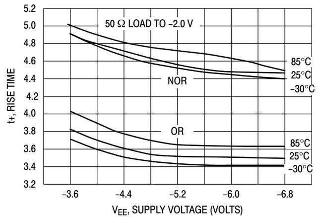
Figure 13. Typical Rise Time (10% to 90%) vs. Temperature and Supply Voltage (MECL 10K)
