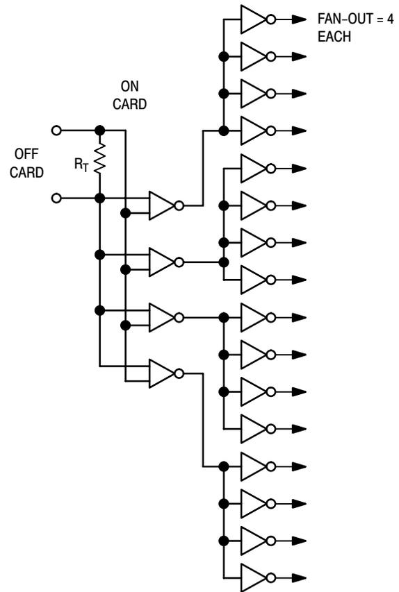
**Figure 36. 64 Fanout Clock Distribution (Proper Termination Required)**
