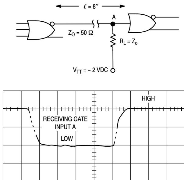
**Figure 2. Properly Terminated Transmission Line (Ground Plane Added)**
