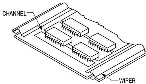
**Figure 25. Channel/Wiper Heatsinking on Double Layer Board**
