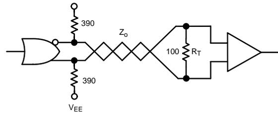
Figure 33. Twisted Pair Line Driver/Receiver
