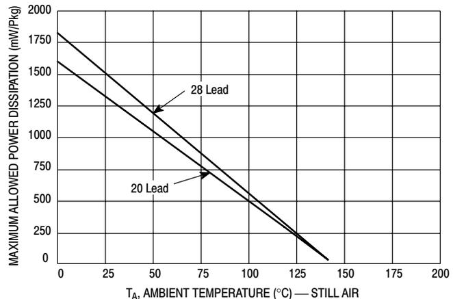
Figure 20. Ambient Temperature Derating Curves (PLCC Package)
