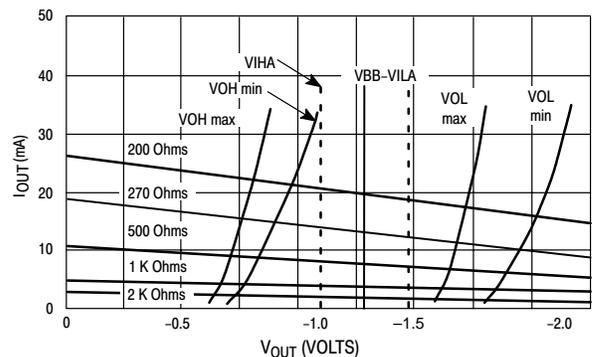
**Figure 17. Output Voltage Levels vs. DC Loading (Load Lines for Termination to  $V_{EE}$  ( $-5.2$  Vdc)  $25^{\circ}\text{C}$ )**
