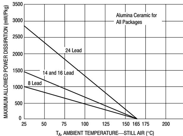
Figure 18. Ambient Temperature Derating Curves (Ceramic Dual-In-Line Package)
