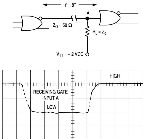
**Figure 2. Properly Terminated Transmission Line (Ground Plane Added)**
