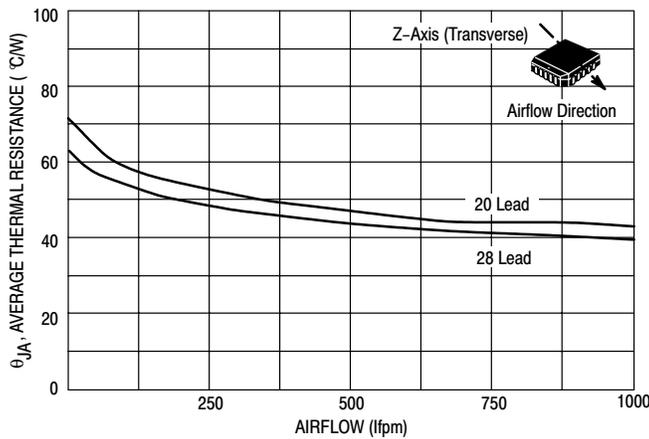
Figure 23. Airflow vs. Thermal Resistance (PLCC Package)
