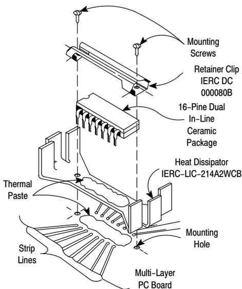
**Figure 26. MECL High-Power Dual-In-Line Package Mounting Method**
