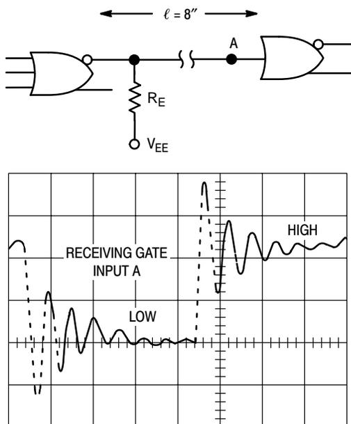
**Figure 1. Underterminated Transmission Line (No Ground Plane Used)**
