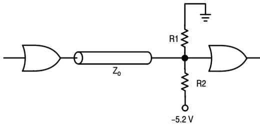
Figure 31. Parallel Termination – Thevenin Equivalent
