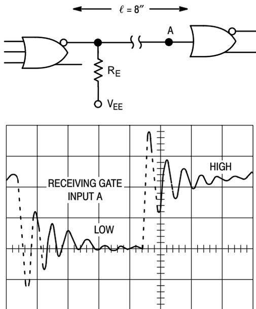
**Figure 1. Unterminated Transmission Line (No Ground Plane Used)**
