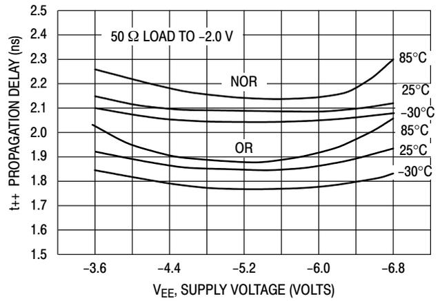
Figure 11. Typical Propagation Delay  $t_{++}$  vs.  $V_{EE}$  and Temperature (MECL 10K)
