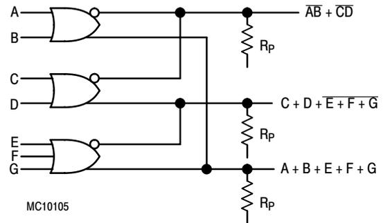
**Figure 37. Use of Wire-OR and Complementary Outputs**
