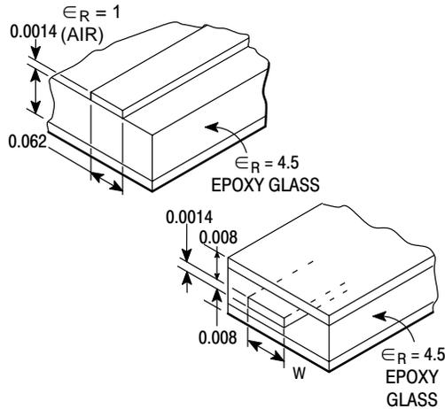
**Figure 35. PC Interconnection Lines for use with MECL**
