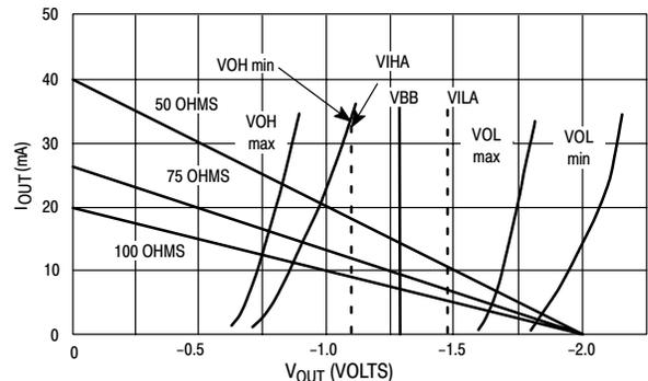
**Figure 16. Output Voltage Levels vs. DC Loading (Load Lines for Termination to  $-2.0$  Vdc  $25^{\circ}\text{C}$ )**
