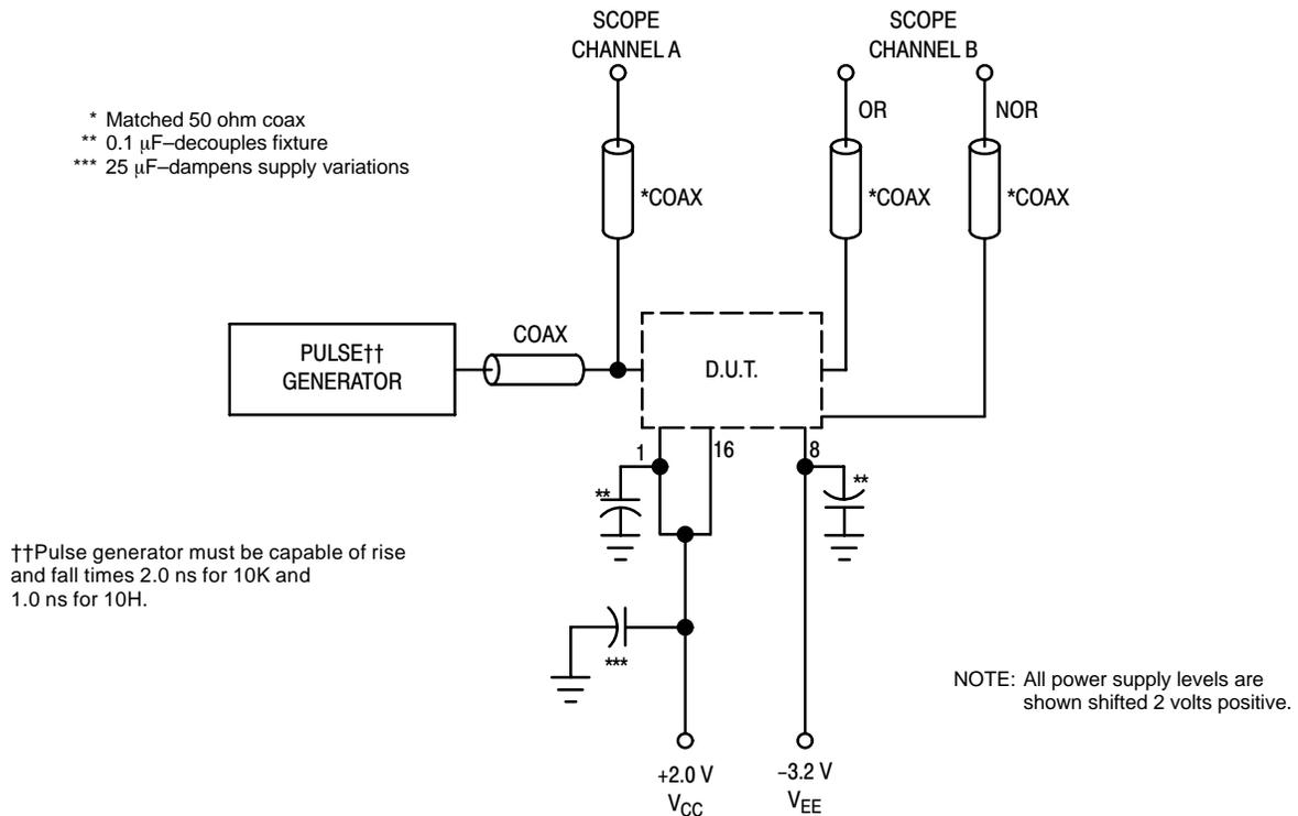
Figure 15. MECL Logic Switching Time Test Setup
