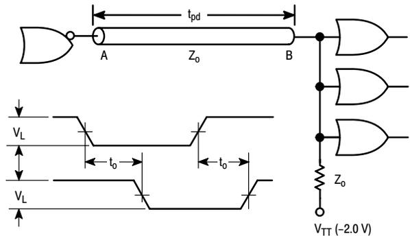
Figure 30. Parallel Terminated Line
