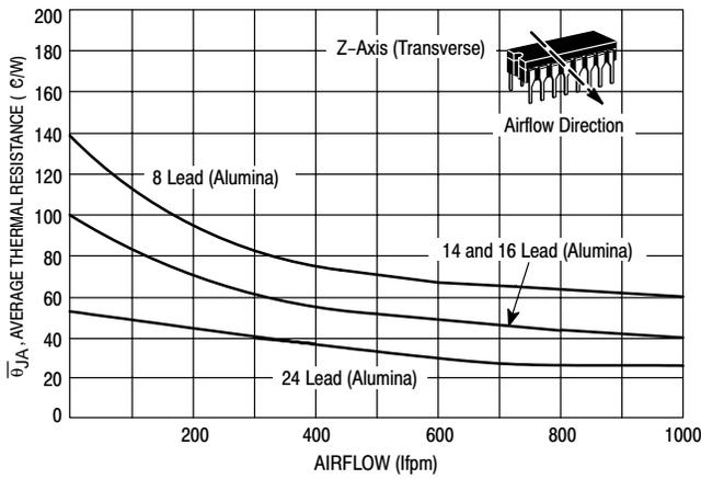
Figure 21. Airflow vs. Thermal Resistance (Ceramic Dual-In-Line Package)
