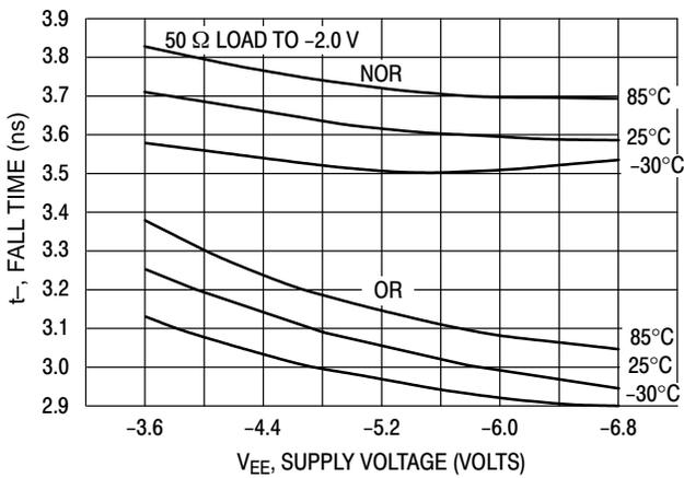
Figure 12. Typical Fall Time (90% to 10%) vs. Temperature and Supply Voltage (MECL 10K)
