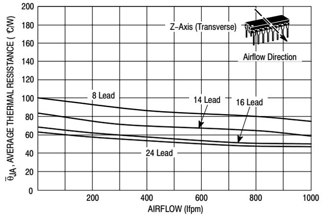
Figure 22. Airflow vs. Thermal Resistance (Plastic Dual-In-Line Package)
