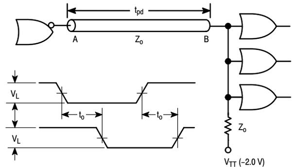
Figure 30. Parallel Terminated Line
