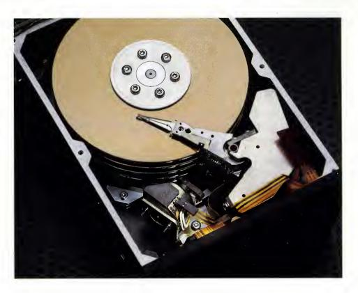
The heads are mounted on a new straight-line arm that is connected to a balanced rotary voice coil actuator. The straight-line design has substantially less mass than other designs, improving accuracy and speed. New high energy magnets in the voice coil further improve performance, resulting in 18-millisecond average seek. A microcomputer controlled, dedicated, closed-loop servo system provides precise positioning control.
