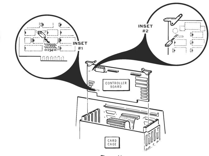
Figure 11 The Winchester disk controller board
