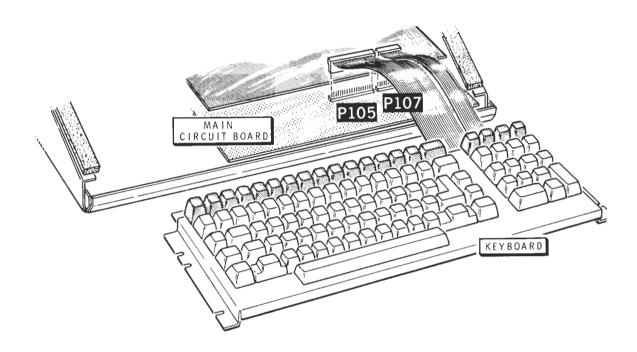
**Pictorial 4-15** Keyboard cable connections Refer to Pictorial 4-16 for the following steps.
