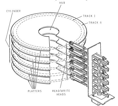
Figure 1 The Ekements of a Hard Disk
