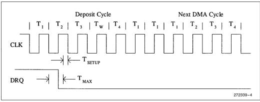
Figure 5. Destination Synchronized DMA Transfer
