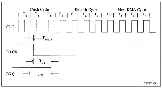
Figure 4. Source Synchronized Transfer
