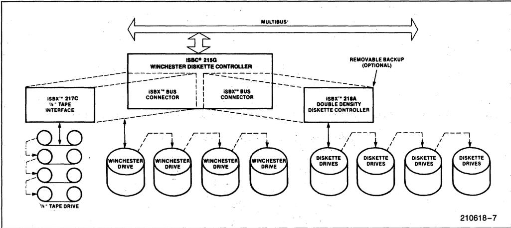
**Figure 3. Subsystem Configuration (with Optional Diskette Backup)**
