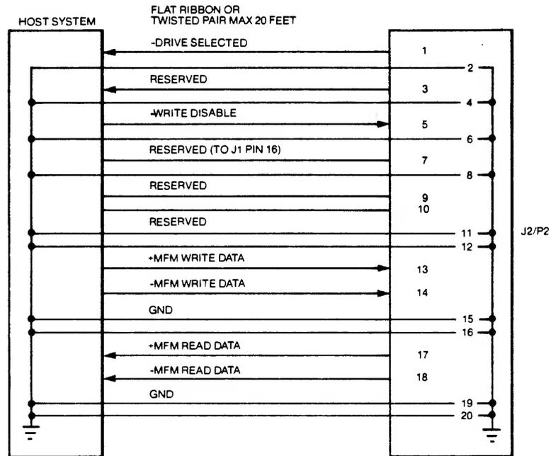
**J2/P2—CONNECTOR PIN ASSIGNMENT**
