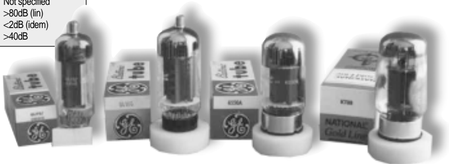
PHOTO 2: 40W beam power tubes.
